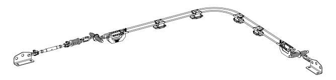
The Travsafe bimaterial version is very similar to the original Travsafe system. It is designed to reduce the higher loading that was generated by the original version. This is done with the use of different kinds of energy absorbers.
